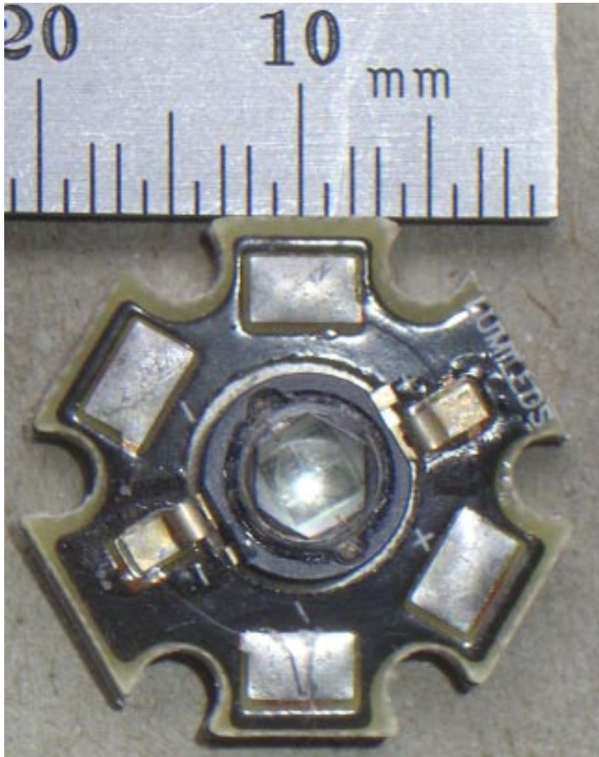
Figure 1: Luxeon V high power LED. Light is emitted by the square active region at the center of the device. This LED emits 1 Watt of light at 470 nm.
